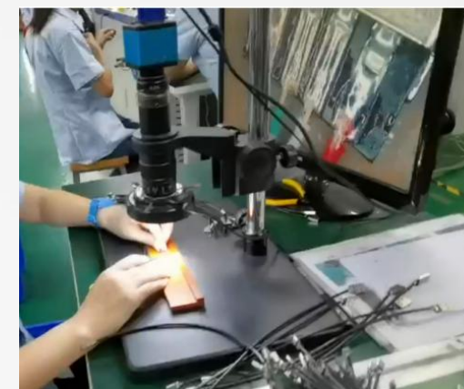
Inspection after soldering
